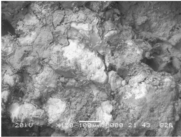
Figure 8 Surface of sintered Ti—50% HA sample, unpolished.
